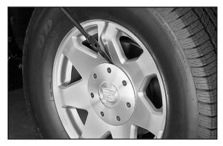
Remove the center cap by placing the chisel end of the wheel wrench in the slot on the wheel and gently prying the cap out.
